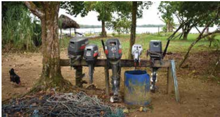
The Travel 1003 (second from the right) electric outboard sitting between two 40 h.p. engines on the resting bench at the end of a journey.
